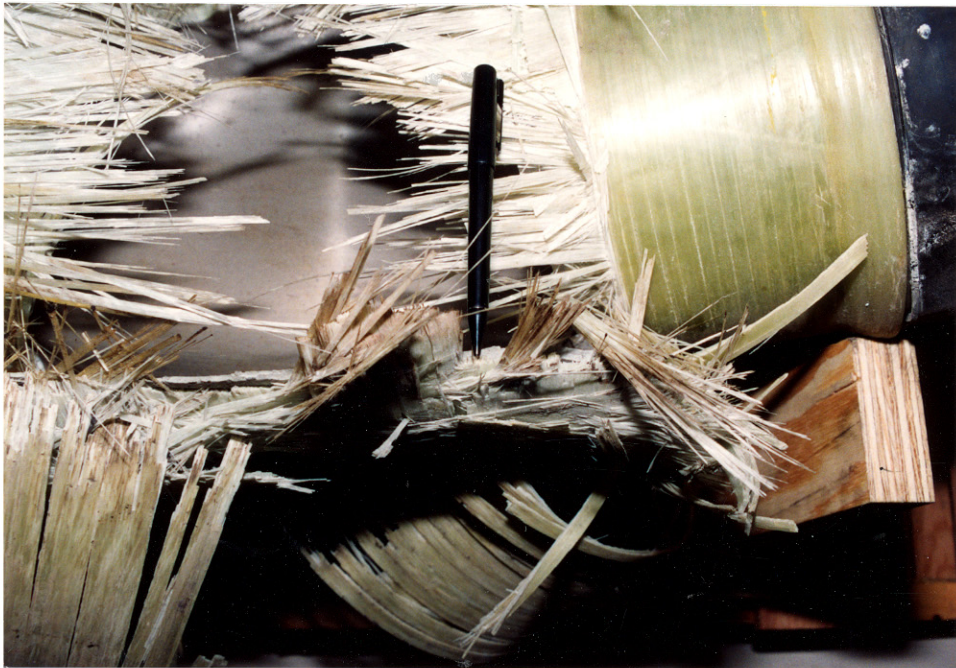
42. Overhead view of the right bottom side of the tank showing the edge of the aluminum tank and composite wrap with the forward end of the tank along the left side of the photograph
